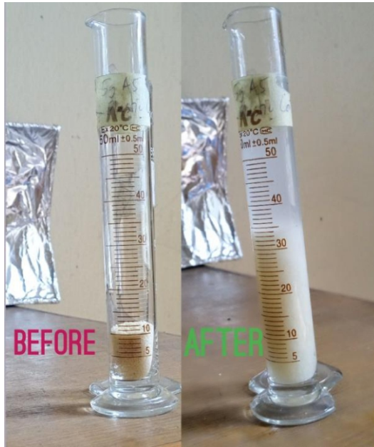
Figure 2: Volume of garri sample in a measuring cylinder before and after swelling.
